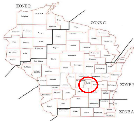
Figure 82.30-1. Frost protection zones.
