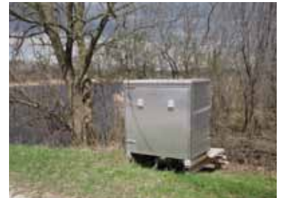
A USGS monitoring station, above, collects water samples for analyzing phosphorus and sediment in Big Green.
