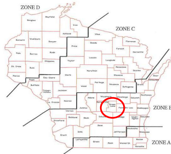
Figure 82.30-1. Frost protection zones.
